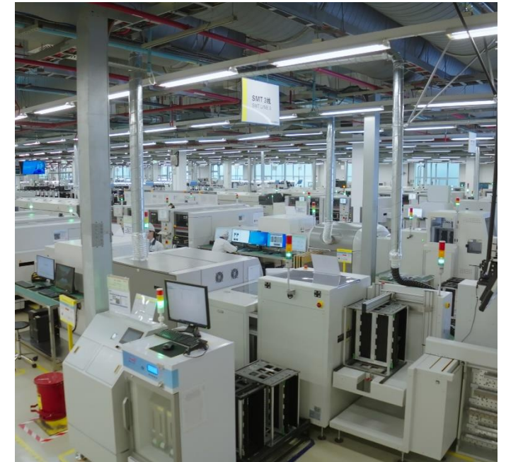
SMT line in Suzhou factory.
